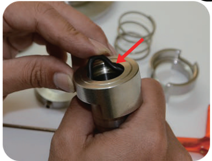
Step1: put O-ring(P12) into the groove of shaft
