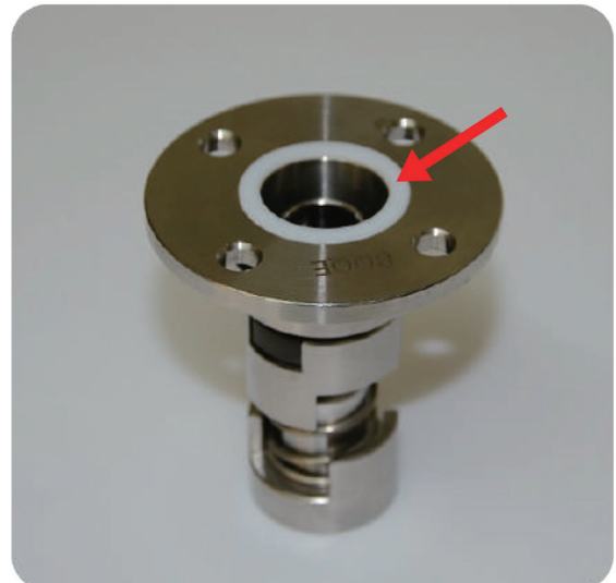
Step10: put the fixed ring on it
