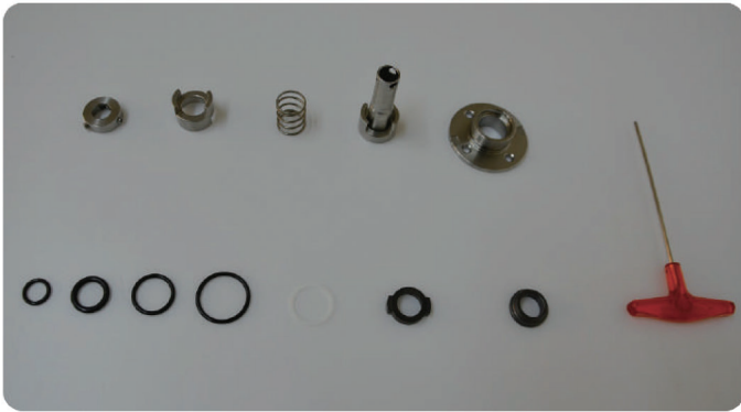
Assemble SB-1,2,3,4,5 SBI-1,2,3,4,5 shaft seal Must be prepared 2.5mm hexagon wrench
