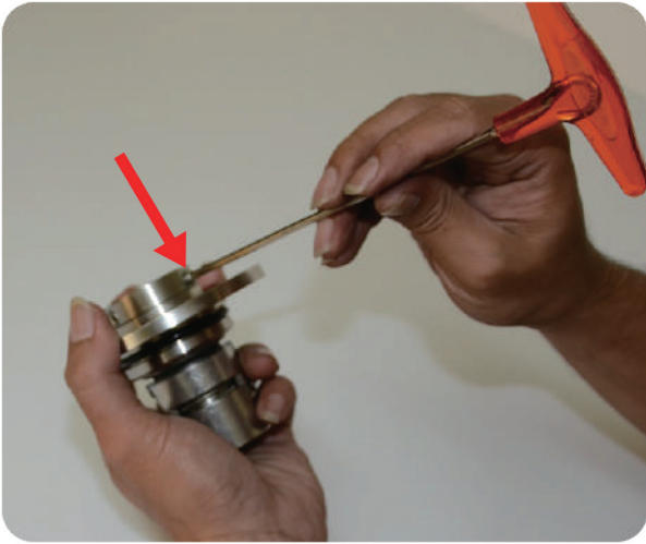
Step1: use 2.5mm hexagon wrench turn on the bolt
