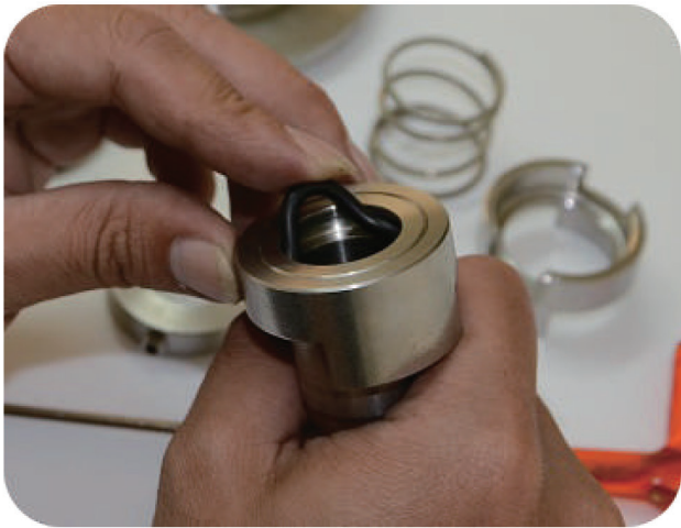
Step9: take out the O- ring (P12) of spindle *suggest using the tool to assist
