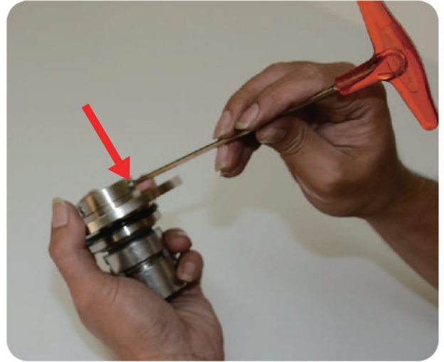
Step11: use 2.5mm hexagon wrench lock the bolt, but it cannot exceed the shaft, just not protrude the hexagon socket head
