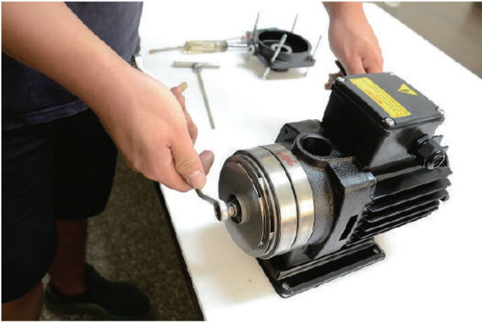
Step6: grasp the universal pliers, use box wrench to take out the lock nut
