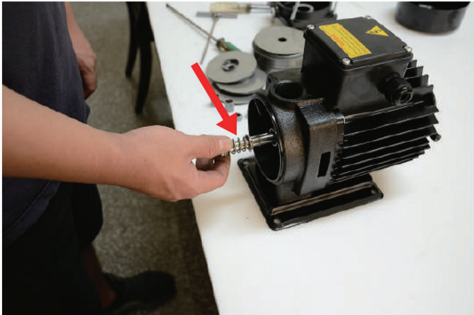
Step2: put the spring in it
