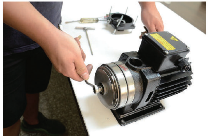
Step9: put the lock nut in it, grasp the universal pliers, use box wrench lock the lock nut
