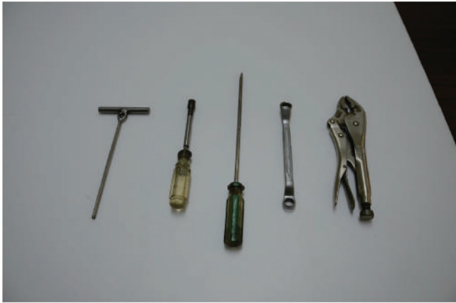
Necessary tools: hexagon, Phillips, flat head screwdriver, box wrench, universal pliers
