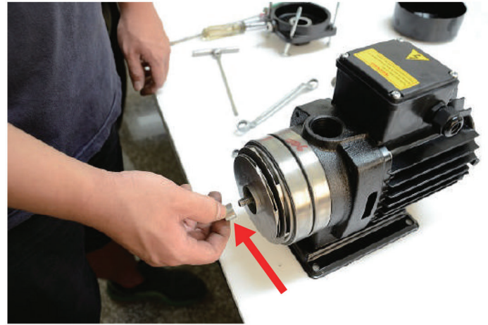
Step7: put the sleeve in it
