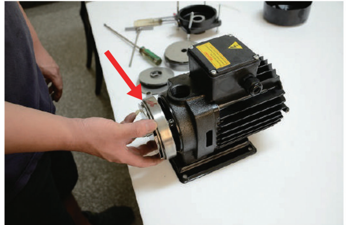
Step3: put the chamber in it
